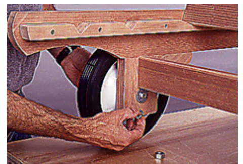
14--After filing away the square shoulder on 1/2-in. carriage bolts, use the bolts as
