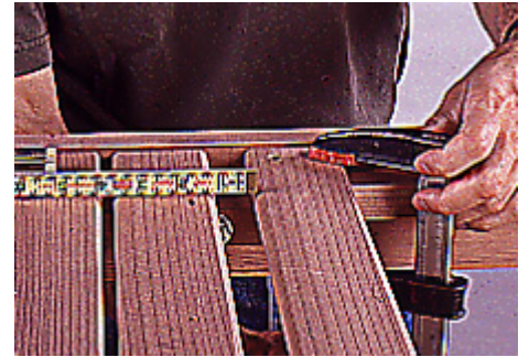
11--Where the backrest joins the fixed seat portion, leave a 1-in. space so the backrest has room to pivot to its highest position.
