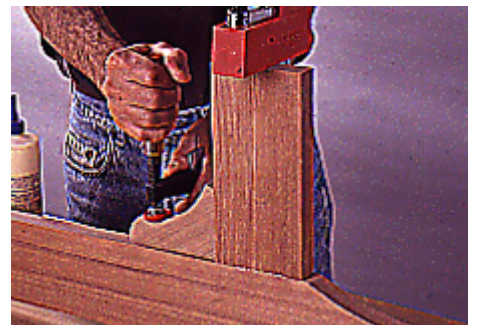
6--When leg/bracket assemblies are finished, join them to the rails. Apply glue to plate and mortise-and-tenon joints, then clamp.
