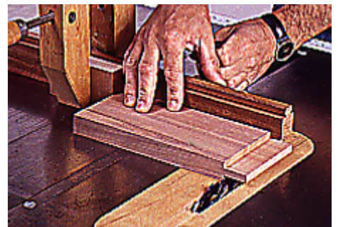
3--Cut the leg tenons with a dado blade and table saw. A stop block clamped to the miter gauge ensures consistent tenon lengths.
