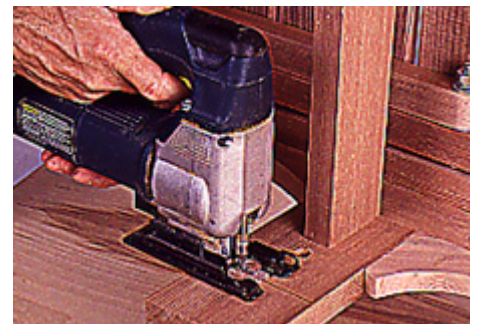
13--To provide clearance for the wheels, cut 3 in. from each rear leg with a sabre saw. Smooth the sawn edges with sandpaper.
