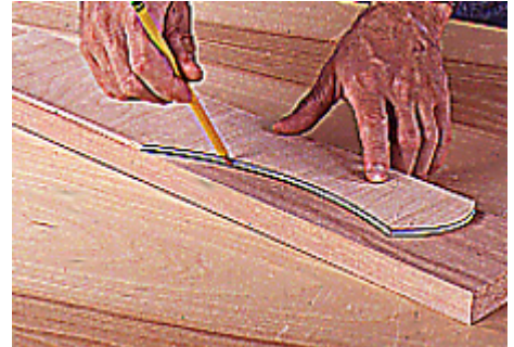
1--Make a 1/4-in.-thick template for the rail-end shape. Then trace the shape onto both ends of each rail blank.
